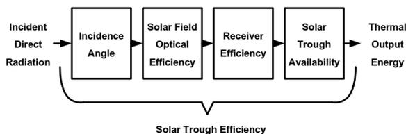
Figure 3: Solar parabolic trough model
