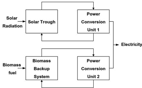
Figure 1: Model of a hybrid power plant with two PCUs
