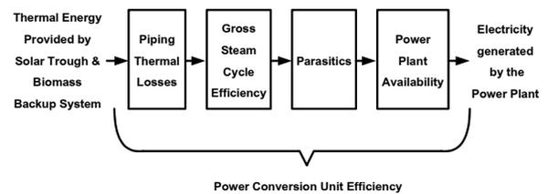
Figure 5: Power Conversion Unit Model
