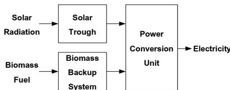
Figure 2: Model of a hybrid power plant with a single PCU
