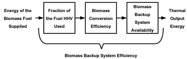
Figure 4: Biomass backup system model
