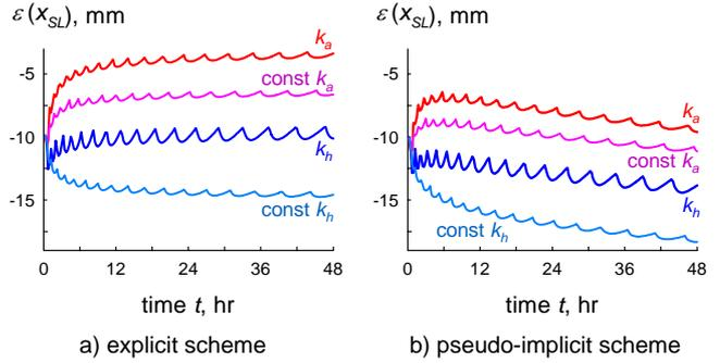
Figure 8 Case 1: Comparisons of ice thickness errors from simulations with constant and varying mean conductivities.
