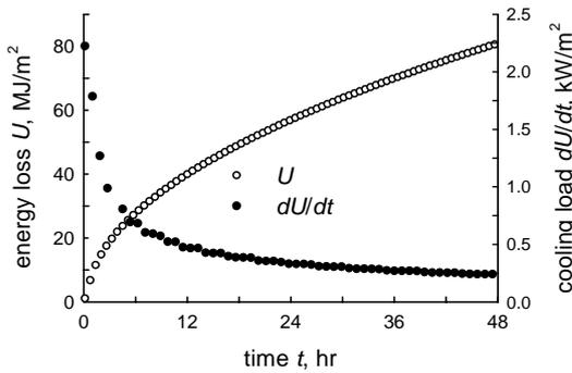
Figure 6 Case 1: Loss of internal energy and cooling loads of the system. The numerical solutions use the explicit/ $k_S$  schemes.
