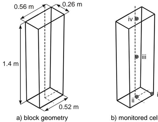
Figure 13 Case 3: Geometry and domain of ice block.
