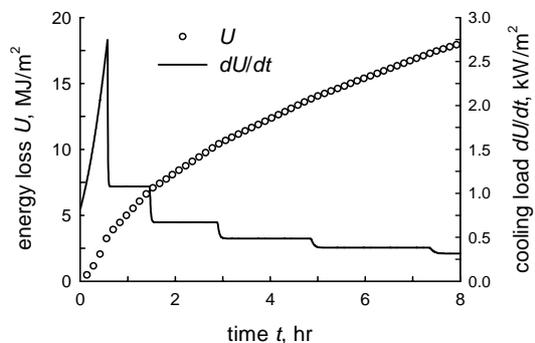
Figure 12 Case 2: Loss of internal energy and the cooling loads of the system.
