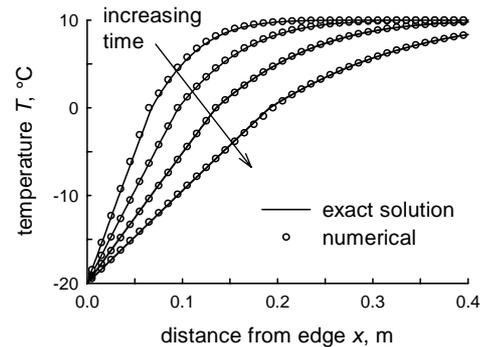
Figure 3 Case 1: Temperature at time 6, 12, 24 and 48 hr. The numerical solutions use the explicit/ $k_S$  schemes.
