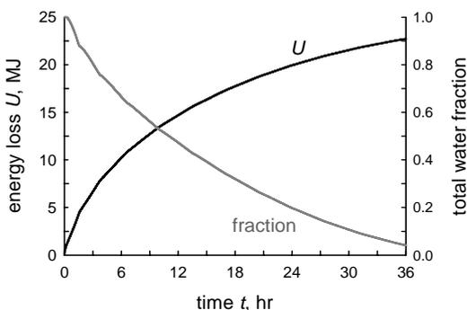
Figure 16 Case 3: Loss of internal energy and ice fraction for the one-quarter block system.
