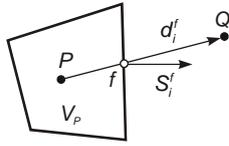
Figure 1 A typical unstructured control volume.
