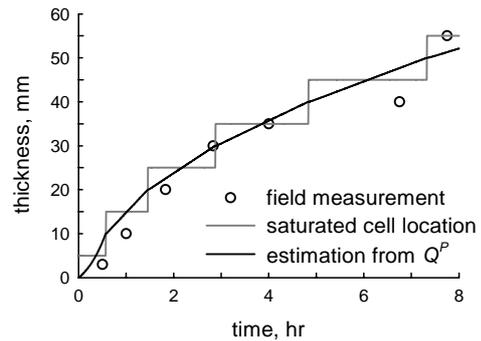
Figure 10 Case 2: Comparison of ice thickness for 1D convective problem. The field data is obtained with slightly different conditions and additional 3.7 mm-thick stainless steel mould [6].
