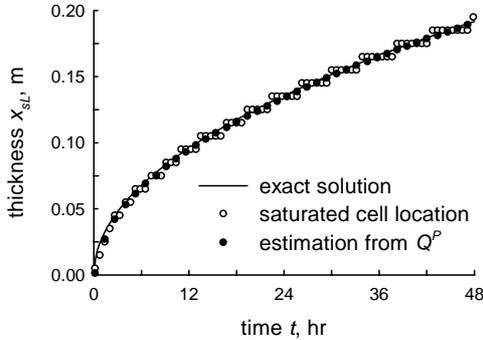
Figure 5 Case 1: Ice thickness. The numerical solutions use the explicit/ $k_S$  schemes.
