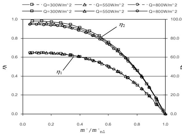
Figure 5: Efficiency Variation with Irradiation
