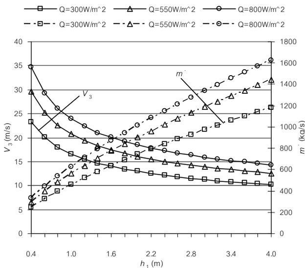
Figure 3: Velocity in Tower Versus Roof Height
