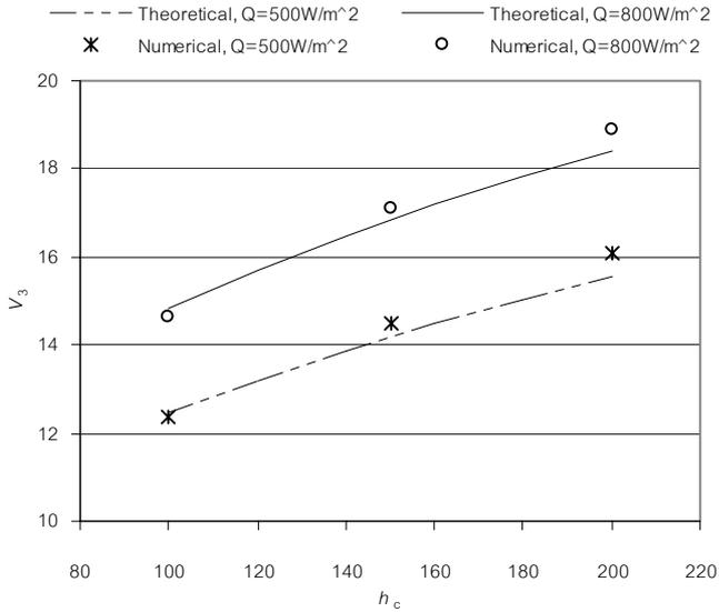
Figure 2: Velocity in Tower Versus Tower height
