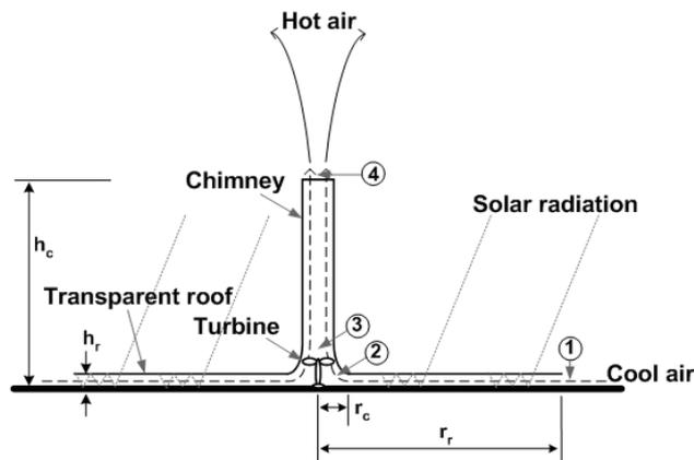
Figure 1: Schematic of Solar Tower
