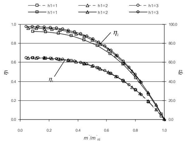
Figure 4: Efficiency Variation with Roof Height
